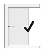
Ensure that there is **no object between the back of the door** and the back stud inside the pocket, which would prohibit the plunger on the *EZ-Closer* from being fully depressed (see diagram). The pocket back stud and back edge of door must be plumb allowing the gap between door and back stud to be parallel.
