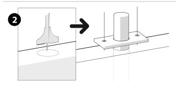
Using a **1 inch spade bit**, bore a hole to the depth of **3.75 inches** (the length of the *EZ-Closer* cylinder). Firmly push the *EZ-Closer* into the drilled hole and secure with the two screws provided (screws must be counter sunk). Now your door is ready to be fitted.
